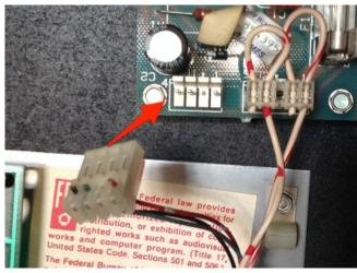
2. Plug harness into board and plug the original connector into the harness.
