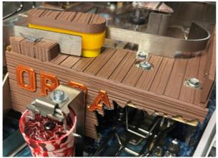
15. insert the railing into the small recesses of the vertical plastic, with the round side of the railing facing the player
