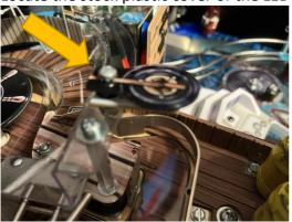
4. unscrew the plastic with a Phillips screwdriver, holding the lock nut from below with a small pair of pliers
