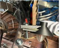
9. now insert the screw through the hole in the ramp. from the underside, place the spacer on the bolt and screw on the lock nut
