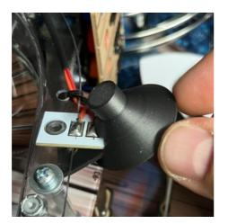
7. now take the sculpted bulb and press it firmly onto the LED from the front until it goes no further. hold the LED board at a slight angle through the lampshade so that you can press on the bulb more easily
