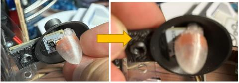
8. take the lamp cover and place it on the led board. insert the screw from above through the lamp cover, led board and lamp
