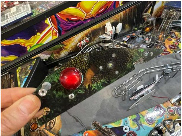
Mount the aluminium hexa (goes on one of the three holes which maintains the helipad), respect the good one:
