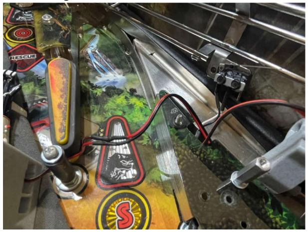
First remove the plastic hexagonal rod placed on the grey helicopter platform. It was placed on the platform of the helicopter in order to see where it was positioned. Don't hesitate to pull hard on it to remove it. You won't break anything  $\cong$ .
