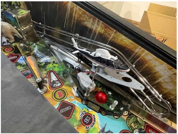
Mount the platform of the helicopter thru the iron rode in the correct hole:
