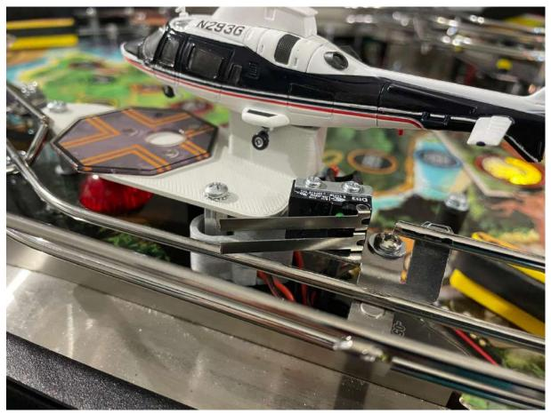
All you have to do is pass the cable coming from our microswitch through the playfield, passing through the same small hole as the microswitch cable which is fitted as standard on your pinball machine. Once the cable has been passed, lift your playfield again and make the connection to the other small blue connector remaining available on the small replacement card that you have attached.
