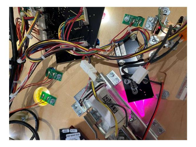
Install our wire between the white connector of red flasher. Respect the color of the wire when you connect the connector. Red electrical wire goes to the red electrical wire:
