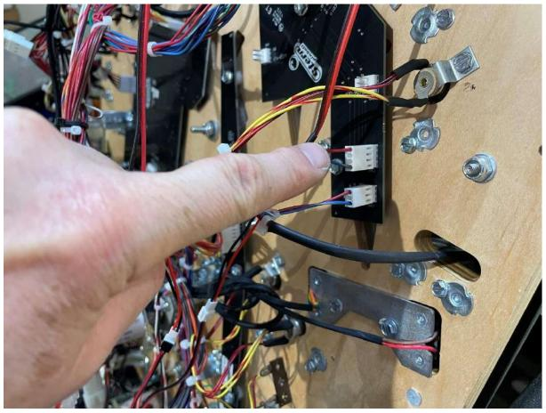
Plug our wire. Respect the correct positioning of the connector (red at the top):
