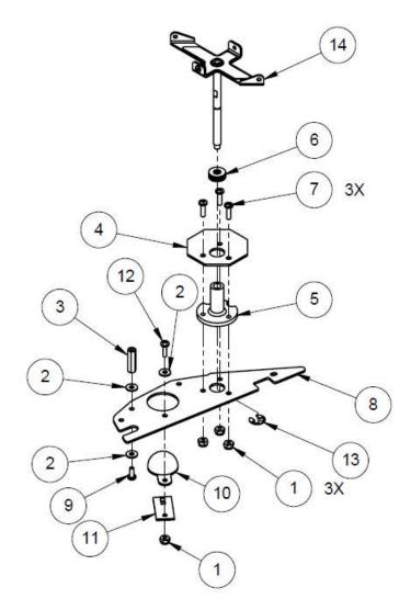
For the PRO machine here it is the plastic assembly:
