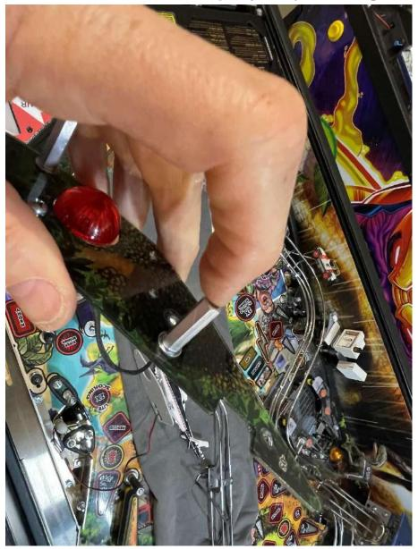
Put again your Helipad ramp on the corridor and pass the wire of it in the triangular hole as you can see in the photo.
