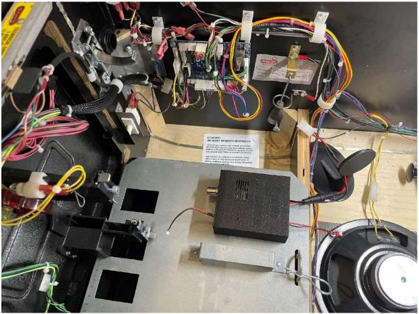
You take the 12v here in the first connector of coindoor card. Name "ticket". Respect the correct pin (x5):
