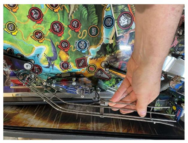
To remove the plastic of the 2D helicopter you have two screws to unscrew:
