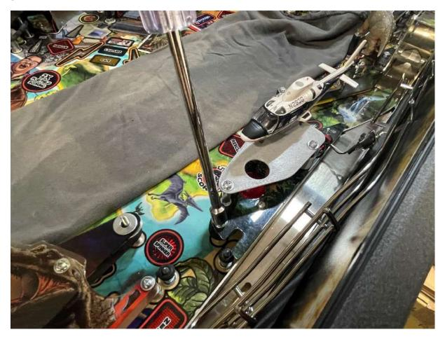
Screw the aluminium hexa (the small one of all) which maintains the ramp:
