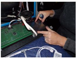
4A.(Stock Speakers) Place the LED Light frame on top of the grill making sure that the screw holes are (UP) and that the lead wire coming off is near the bottom corner of your DMD. Once in position, replace the speaker and screw in all 4 corners using the longer provided screws with the kit. Remember to hook the ground strap back on. (IF YOU HAVE UPGRADED SPEAKERS INSTALLED SEE NEXT PAGE)
