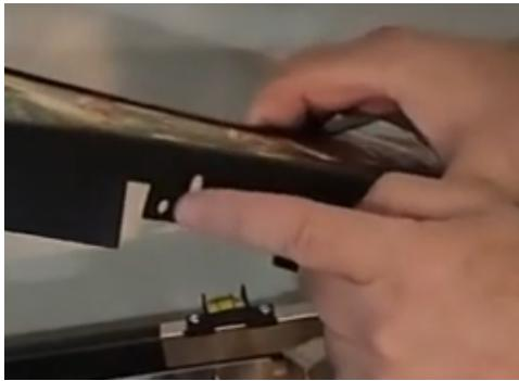
**(5B)** Hold nuts in with finger and tighten screws.
