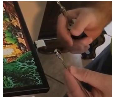
20. When apron is in position, use supplied bolts and put through the holes in the playfield hanging brackets. Hold the lock nut under the apron with a finger. Tighten screw with a screwdriver until lock nut starts to spin. Now use an  $11/32^{\text{nd}}$  inch wrench to secure the nut and tighten the screw. **These need to be tightened completely** or if they come forward, they will get under your lockdown receiver bar, and you will have difficulties removing the playfield later. **(5B) (5C)**
