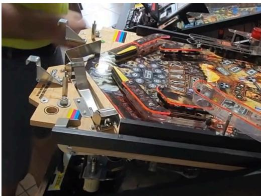
(2B) These are the 4 bolts that need to be removed but leave brackets in place. The white light panel goes over those brackets.
