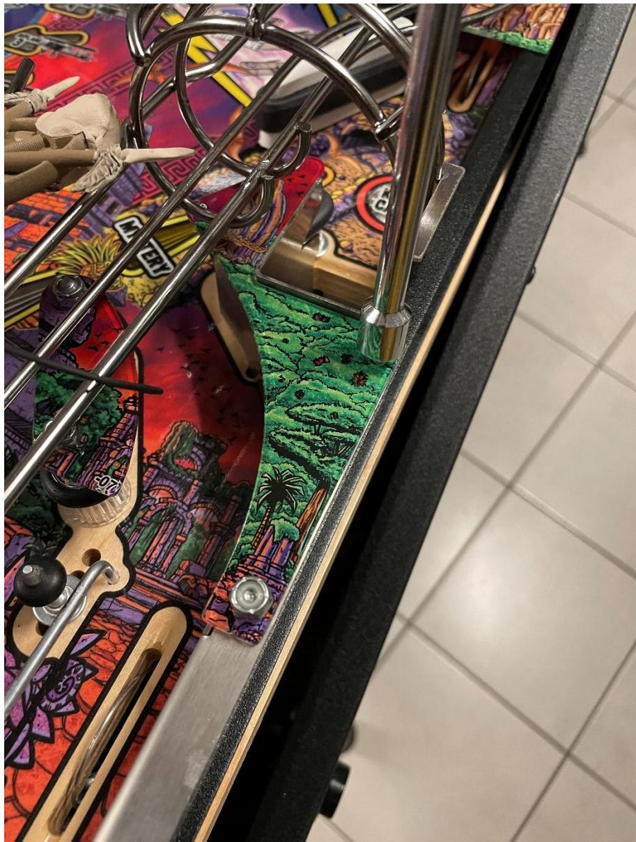
**To remove this plastic you need to unscrew the two nuts with a suitable wrench.**
