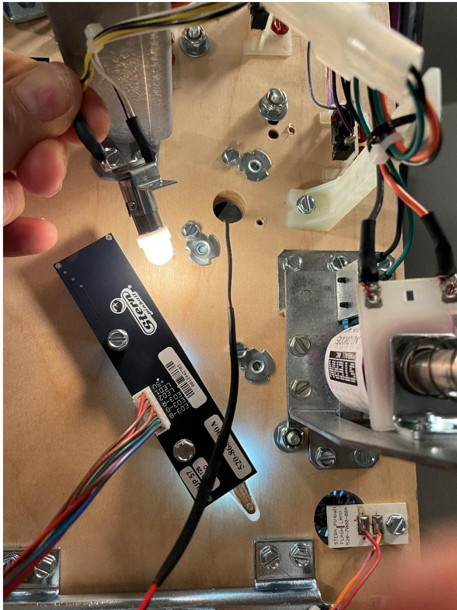
**Once unscrewed, you can pass the cable of your Dreamcatcher through the hole you see. Of course, to pass this cable you have to lower your playfield again and pass the cable through the hole located just below the plastic number - 07.**
