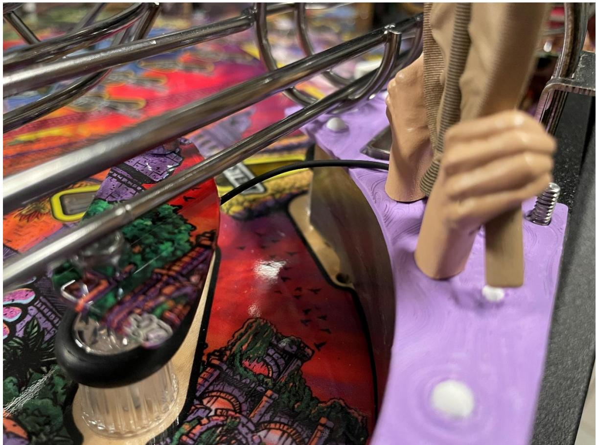
**In the following picture you can clearly see the cable near the special bulb that we placed in place of the existing bulb. This special bulb allows us to supply 5v and thus light up the red eyes of your Dreamcatcher.**
